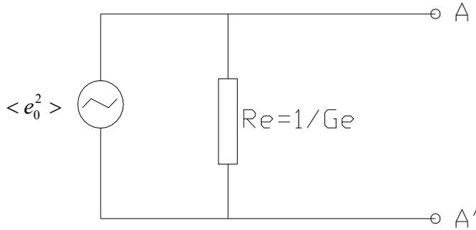
Figure 2.1 Equivalent noise circuits at non-zero bias
