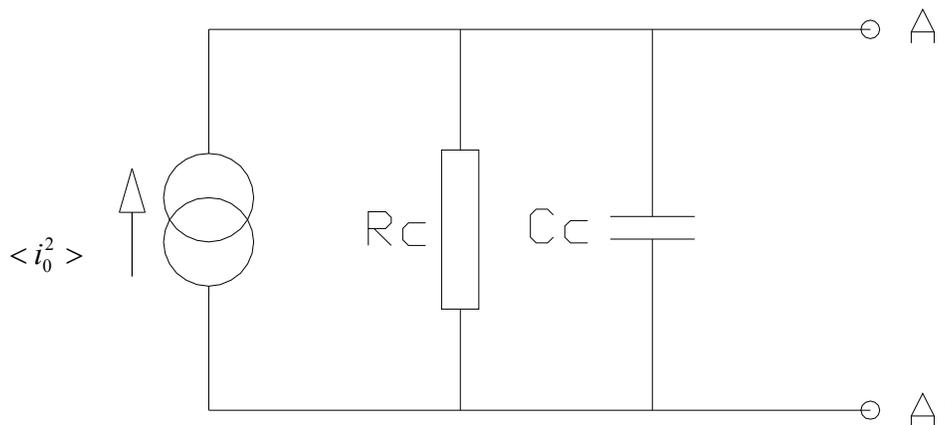
Figure 1.3 Equivalent noise circuit at zero bias considering the barrier capacitance
