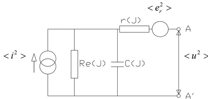
Figure 2.2 Equivalent noise circuits of the structure with a potential barrier
