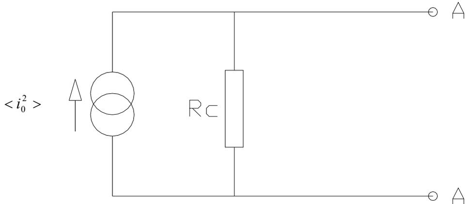
Figure 1.2 Equivalent noise circuit at zero bias
