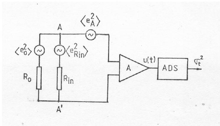
Figure 6.2 Noise Measurement Circuit by Statistical Distribution
